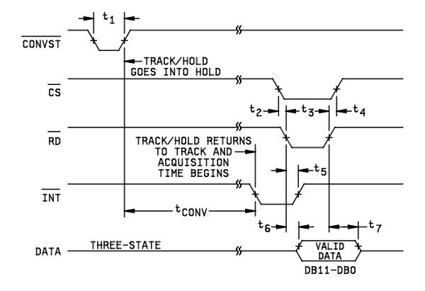
FIGURE 2. Timing waveforms.
